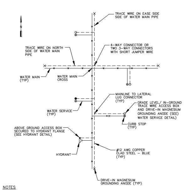
WRE SHOWN AWAY FROM PIPE FOR CLARITY. WIRE SHALL BE INSTALLED ON THE BOTTOM SIDE OF THE PIPE BELOW THE SPRING LINE. THE WIRE SHALL BE FASTENED TO THE PIPE TAPE OR PLASTIC TIES AT 5' INTERVALS.
