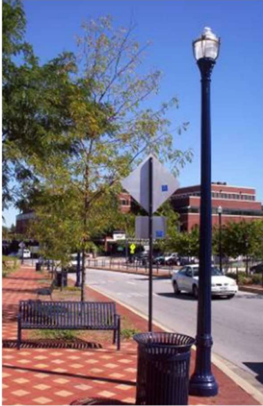
Traditional aluminum fixture with cut-off to address “Night Skies” initiatives in urban areas – 12’-14’
