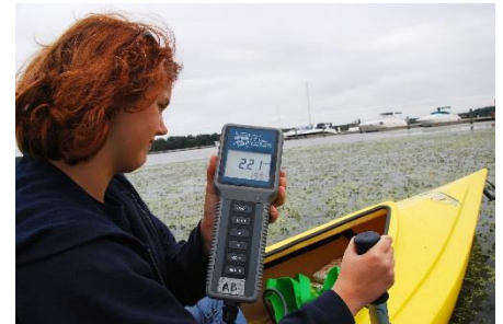
Low dissolved oxygen reading in a bed of submerged aquatic vegetation burdened by macro-algae, summer of 2011. The value of 2.21 mg/liter is well below the minimum standard of 5 mg/liter, and lethal to many fish species.
