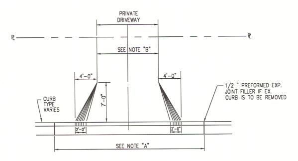
NOTE A: WHERE CURB AND GUTTER EXISTS, REMOVE AND RECONSTRUCT CURB AND GUTTER TO FIRST JOINT ON EITHER SIDE OF ENTRANCE.
