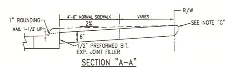
NOTE C: IF PRIVATE DRIVEWAY IS CONCRETE PROVIDE 1/2" PREFORMED EXPANSION JOINT FILLER AT R/W LINE.
