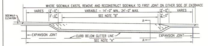
NOTE A: WHERE CURB & GUTTER EXISTS, REMOVE AND RECONSTRUCT CURB & GUTTER TO FIRST JOINT ON EITHER SIDE OF ENTRANCE.
