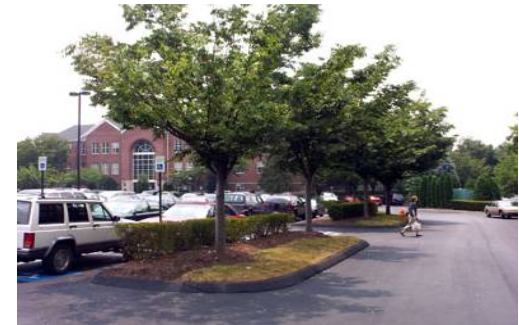
Surface parking should have a landscaped median to separate the driveway from the parking aisle
