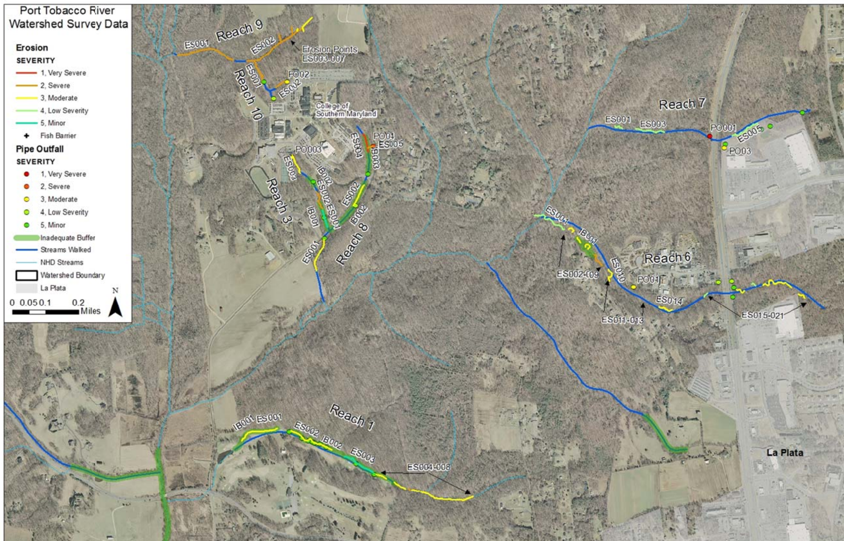
FIGURE 7: SURVEY DATA MAP SHOWING PIPE OUTFALL, EROSION, FISH BARRIER, AND INADEQUATE BUFFER SITES, NOTHERN REACHES
