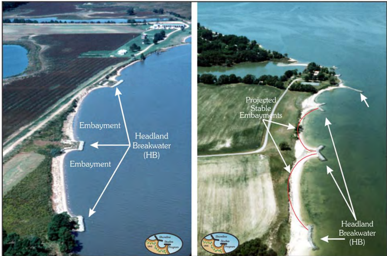
Figure 4-6. Examples of headland breakwaters spaced widely apart to allow adjacent shoreline to erode toward a dynamic equilibrium. This is a cost-effective shoreline management strategy when infrastructure is not threatened by the upland erosion between the structures. From Hardaway and Byrne (1999).
