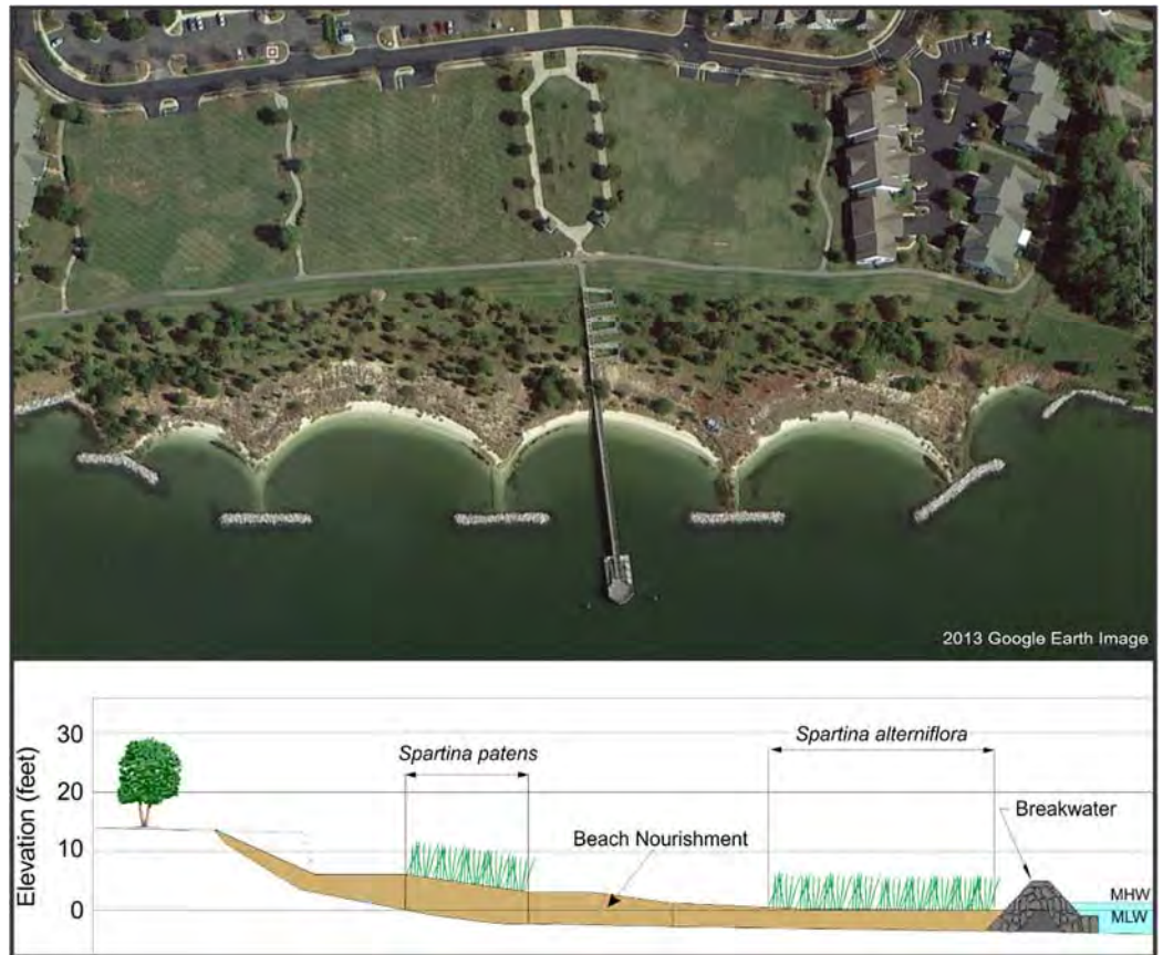
Figure 4-3. Image from Google Earth showing a breakwater installation (top) and a typical breakwater cross-section (bottom).
